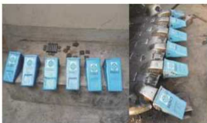
Digger Teeth developed with ADI technology
