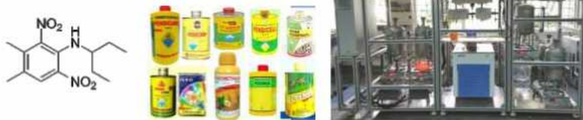
Figure: (Left) Molecular structure of pendimethalin, (Middle) Various commercially available pendimethalin formulation brands from India (taken from internet), (Right). The continuous pilot plant established at CSIR-NCL for synthesis of pendimethalin at 50 kg/day.
