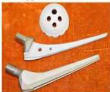
Plasma spray HAp coated hip joint stems and shell
