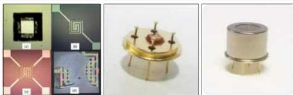
Gas sensor chip and its package
