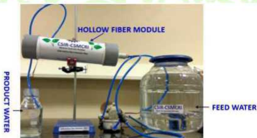
Lab-scale Hollow fiber module testing system
