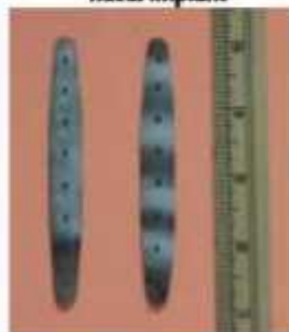
Plasma spray HAp coated nasal implant
