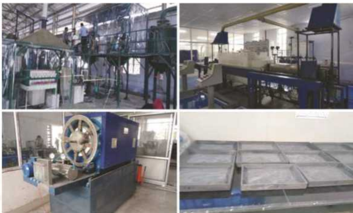
100 Kg/day scale tungsten recycling pilot plant at CSIR-NML & Tungsten (W) powder produced in large scale
